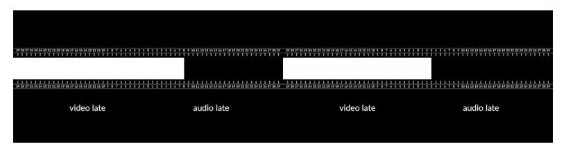
In this combined video output, the original video is on the left and the captured video on the right. The frame counter at the moment this snapshot was taken in the example above is at +8 frames and the counter for the captured video is at +3 frames. The difference between the two demonstrates that the software has 5 frames of latency from output to output in this specific scenario.
