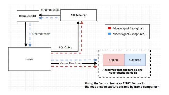
The converter that we use for testing is the <u>Bird dog studio 2</u>: Which has a claimed latency of 1 frame when going from SDI to NDI.
